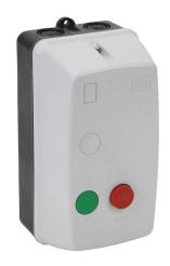
WEG Electric PESWS series manual motor starter, pushbutton, 18A, 2-pole, 208-240 VAC (60Hz)/180-208 VAC (50Hz) coil voltage, thermal overload, 10.0-15.0.A Adjustable, NEMA 4/4X.
