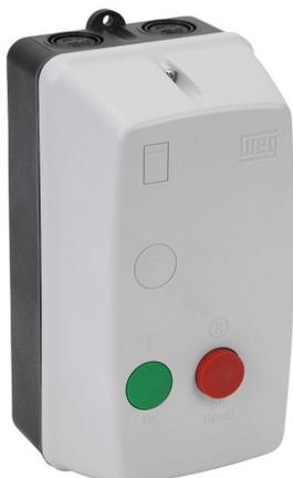
WEG Electric PESWS series manual motor starter, pushbutton, 18A, 2-pole, 120 VAC (50/60Hz) coil voltage, thermal overload, 11.0-17.0.A Adjustable, NEMA 4/4X.
