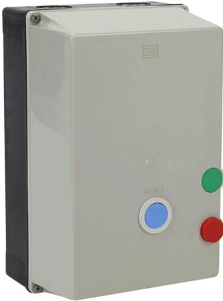
WEG Electric PESW series manual motor starter, pushbutton, 80A, 3-pole, 208-240 VAC (60Hz)/180-208 VAC (50Hz) coil voltage, thermal overload, 57.0-70.0A adjustable, NEMA 4/4X.
