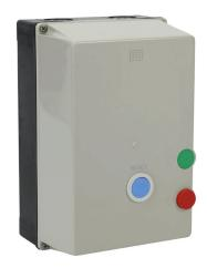
WEG Electric PESW series manual motor starter, pushbutton, 80A, 3-pole, 120 VAC (50/60Hz) coil voltage, thermal overload, 63.0-80.0A adjustable, NEMA 4/4X.
