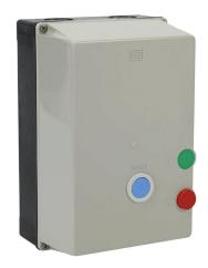
WEG Electric PESW series manual motor starter, pushbutton, 65A, 3-pole, 208-240 VAC (60Hz)/180-208 VAC (50Hz) coil voltage, thermal overload, 50.0-63.0A adjustable, NEMA 4/4X.
