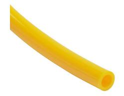
HydroMode potable water tubing, polyethylene, yellow, 5/32in (4mm) outside diameter, 0.106in inside diameter, NSF/ANSI 61, 100ft package.
