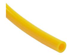
HydroMode potable water tubing, polyethylene, yellow, 5/32in (4mm) outside diameter, 0.106in inside diameter, NSF/ANSI 61, 1000ft reel.
