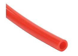
HydroMode potable water tubing, polyethylene, red, 5/32in (4mm) outside diameter, 0.106in inside diameter, NSF/ANSI 61, 500ft reel.
