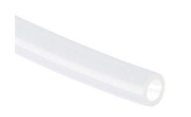
HydroMode potable water tubing, polyethylene, natural, 5/32in (4mm) outside diameter, 0.106in inside diameter, NSF/ANSI 61, 1000ft reel.
