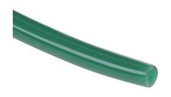
HydroMode potable water tubing, polyethylene, green, 5/32in (4mm) outside diameter, 0.106in inside diameter, NSF/ANSI 61, 100ft package.
