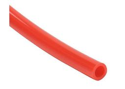
HydroMode potable water tubing, polyethylene, red, 5/16in (8mm) outside diameter, 0.236in inside diameter, NSF/ANSI 61, 500ft reel.
