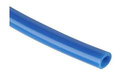
HydroMode potable water tubing, polyethylene, blue, 5/16in (8mm) outside diameter, 0.236in inside diameter, 500ft reel.
