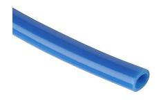
HydroMode potable water tubing, polyethylene, blue, 5/16in (8mm) outside diameter, 0.236in inside diameter, NSF/ANSI 61, 1000ft reel.
