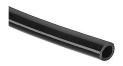
HydroMode potable water tubing, polyethylene, black, 5/16in (8mm) outside diameter, 0.236in inside diameter, NSF/ANSI 61, 500ft reel.
