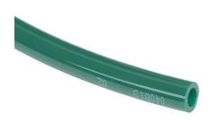
HydroMode potable water tubing, polyethylene, green, 3/8in outside diameter, 1/4in inside diameter, NSF/ANSI 61, 500ft reel.
