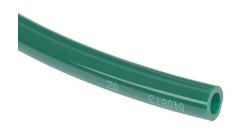
HydroMode potable water tubing, polyethylene, green, 3/8in outside diameter, 1/4in inside diameter, NSF/ANSI 61, 100ft package.
