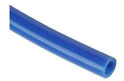
HydroMode potable water tubing, polyethylene, blue, 3/8in outside diameter, 1/4in inside diameter, NSF/ANSI 61, 100ft package.
