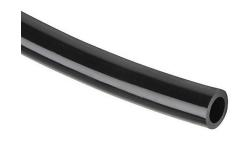
HydroMode potable water tubing, polyethylene, black, 3/8in outside diameter, 1/4in inside diameter, NSF/ANSI 61, 1000ft reel.
