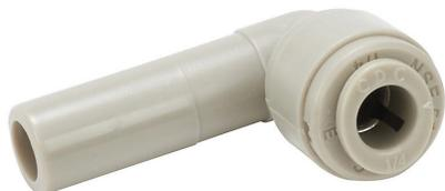
HydroMode potable water push-to-connect fitting, plug-in elbow, acetal body, (1) 3/8in plug-in to (1) 1/4in tube connection(s), NSF/ANSI 61. Package of 5.
