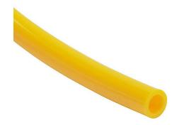
HydroMode potable water tubing, polyethylene, yellow, 1/4in outside diameter, 0.170in inside diameter, NSF/ANSI 61, 500ft reel.
