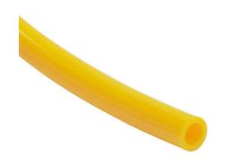
HydroMode potable water tubing, polyethylene, yellow, 1/4in outside diameter, 0.170in inside diameter, NSF/ANSI 61, 100ft package.
