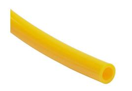
HydroMode potable water tubing, polyethylene, yellow, 1/4in outside diameter, 0.170in inside diameter, NSF/ANSI 61, 1000ft reel.
