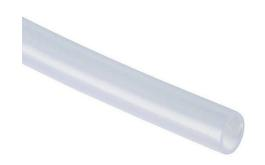
HydroMode potable water tubing, polyethylene, natural, 1/4in outside diameter, 0.170in inside diameter, NSF/ANSI 61, 1000ft reel.
