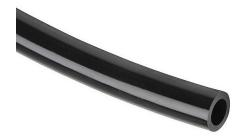
HydroMode potable water tubing, polyethylene, black, 1/4in outside diameter, 0.170in inside diameter, NSF/ANSI 61, 100ft package.
