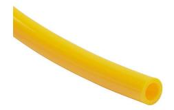
HydroMode potable water tubing, polyethylene, yellow, 1/2in outside diameter, 3/8in inside diameter, NSF/ANSI 61, 100ft package.
