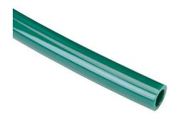
HydroMode potable water tubing, polyethylene, green, 1/2in outside diameter, 3/8in inside diameter, NSF/ANSI 61, 500ft reel.
