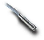
AutomationDirect inductive proximity sensor, tubular, 5mm diameter x 25mm body, stainless steel housing, PNP, N.O. output, 1.5mm sensing distance, flush, 3 kHz switching frequency, IP67, pigtail.
