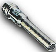
AutomationDirect inductive proximity sensor, tubular, 5mm diameter x 38mm body, stainless steel housing, PNP, N.O. output, 0.8mm sensing distance, flush, 5 kHz switching frequency, IP67, 3-pin M8 quick-disconnect.
