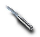
AutomationDirect inductive proximity sensor, tubular, 5mm diameter x 25mm body, stainless steel housing, PNP, N.O. output, 0.8mm sensing distance, flush, 5 kHz switching frequency, IP67, pigtail.
