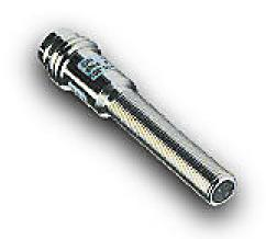
AutomationDirect inductive proximity sensor, tubular, 5mm diameter x 38mm body, stainless steel housing, NPN, N.O. output, 1.5mm sensing distance, flush, 3 kHz switching frequency, IP67, 3-pin M8 quick-disconnect.
