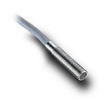
AutomationDirect inductive proximity sensor, tubular, 5mm diameter x 25mm body, stainless steel housing, NPN, N.O. output, 1.5mm sensing distance, flush, 3 kHz switching frequency, IP67, pigtail.
