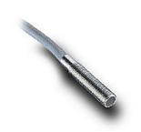
AutomationDirect inductive proximity sensor, tubular, 5mm diameter x 25mm body, stainless steel housing, NPN, N.O. output, 0.8mm sensing distance, flush, 5 kHz switching frequency, IP67, pigtail.
