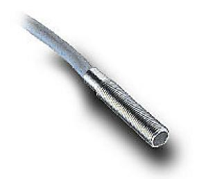
AutomationDirect inductive proximity sensor, tubular, 5mm diameter x 25mm body, stainless steel housing, NPN, N.O. output, 0.8mm sensing distance, flush, 5 kHz switching frequency, IP67, pigtail.
