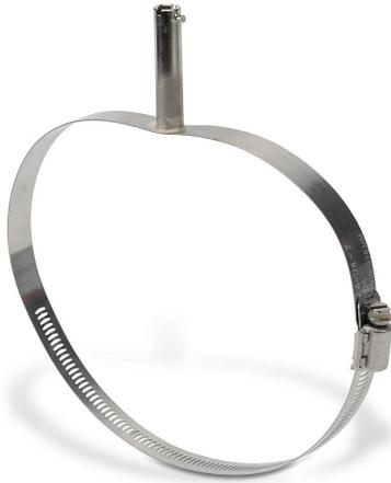
ProSense pipe clamp with bayonet adapter, 4-1/8 to 7in adjustable diameter, 2in bayonet length, 7/16in bayonet outside diameter, 9/32in bayonet inside diameter. For use with adjustable immersion sensors.
