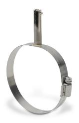
ProSense pipe clamp with bayonet adapter, 3-5/16 to 4-1/4in adjustable diameter, 2in bayonet length, 7/16in bayonet outside diameter, 9/32in bayonet inside diameter. For use with adjustable immersion sensors.
