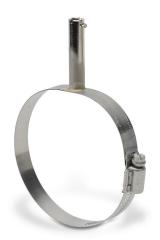
ProSense pipe clamp with bayonet adapter, 3-5/16 to 4-1/4in adjustable diameter, 2in bayonet length, 7/16in bayonet outside diameter, 9/32in bayonet inside diameter. For use with adjustable immersion sensors.
