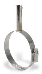
ProSense pipe clamp with bayonet adapter, 2-1/16 to 3in adjustable diameter, 2in bayonet length, 7/16in bayonet outside diameter, 9/32in bayonet inside diameter. For use with adjustable immersion sensors.
