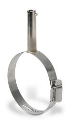
ProSense pipe clamp with bayonet adapter, 2-1/16 to 3in adjustable diameter, 2in bayonet length, 7/16in bayonet outside diameter, 9/32in bayonet inside diameter. For use with adjustable immersion sensors.
