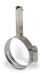
ProSense pipe clamp with bayonet adapter, 1-1/16 to 2in adjustable diameter, 2in bayonet length, 7/16in bayonet outside diameter, 9/32in bayonet inside diameter. For use with adjustable immersion sensors.
