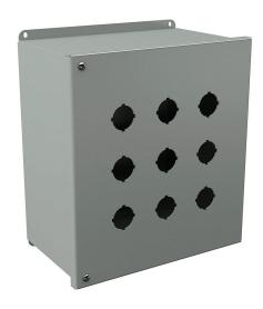
Wiegmann pushbutton enclosure, 9 holes, 30mm, NEMA 12/13, 11 x 10 x 6in (HxWxD), wall mount, carbon steel, ANSI 61 gray, powder coat finish, hinged screw cover, subpanel included.
