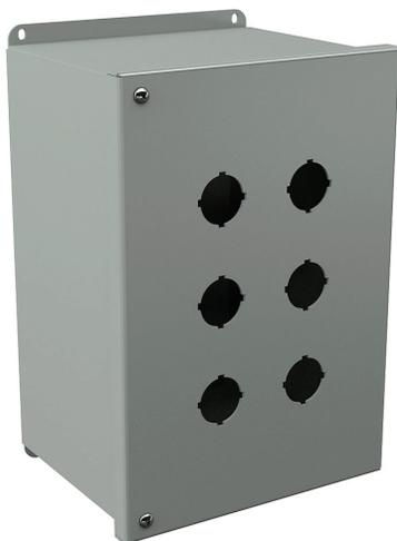
Wiegmann pushbutton enclosure, 6 holes, 30mm, NEMA 12/13, 11 x 8 x 6in (HxWxD), wall mount, carbon steel, ANSI 61 gray, powder coat finish, hinged screw cover, subpanel included.
