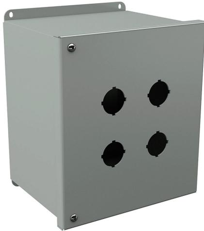
Wiegmann pushbutton enclosure, 4 holes, 30mm, NEMA 12/13, 9 x 8 x 6in (HxWxD), wall mount, carbon steel, ANSI 61 gray, powder coat finish, hinged screw cover, subpanel included.
