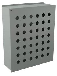
Wiegmann pushbutton enclosure, 42 holes, 30mm, NEMA 12/13, 21 x 18 x 6in (HxWxD), wall mount, carbon steel, ANSI 61 gray, powder coat finish, hinged screw cover, subpanel included.
