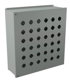
Wiegmann pushbutton enclosure, 36 holes, 30mm, NEMA 12/13, 19 x 18 x 6in (HxWxD), wall mount, carbon steel, ANSI 61 gray, powder coat finish, hinged screw cover, subpanel included.
