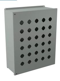
Wiegmann pushbutton enclosure, 30 holes, 30mm, NEMA 12/13, 19 x 15 x 6in (HxWxD), wall mount, carbon steel, ANSI 61 gray, powder coat finish, hinged screw cover, subpanel included.
