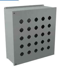
Wiegmann pushbutton enclosure, 25 holes, 30mm, NEMA 12/13, 16 x 15 x 6in (HxWxD), wall mount, carbon steel, ANSI 61 gray, powder coat finish, hinged screw cover, subpanel included.
