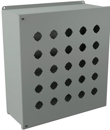
Wiegmann pushbutton enclosure, 25 holes, 30mm, NEMA 12/13, 16 x 15 x 6in (HxWxD), wall mount, carbon steel, ANSI 61 gray, powder coat finish, hinged screw cover, subpanel included.
