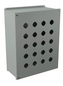
Wiegmann pushbutton enclosure, 20 holes, 30mm, NEMA 12/13, 16 x 13 x 6in (HxWxD), wall mount, carbon steel, ANSI 61 gray, powder coat finish, hinged screw cover, subpanel included.
