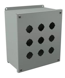
Wiegmann pushbutton enclosure, 9 holes, 30mm, NEMA 4/12/13, 10 x 9 x 5in (HxWxD), wall mount, carbon steel, ANSI 61 gray, powder coat finish, screw cover.
