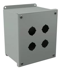
Wiegmann pushbutton enclosure, 4 holes, 30mm, NEMA 4/12/13, 7 x 6 x 5in (HxWxD), wall mount, carbon steel, ANSI 61 gray, powder coat finish, screw cover.
