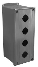
Wiegmann pushbutton enclosure, 4 holes, 30mm, NEMA 4/4X/12/13, 10 x 4 x 5in (HxWxD), wall mount, 304 stainless steel, No. 3 intermediate polished finish, screw cover.
