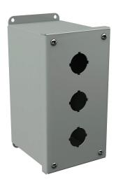
Wiegmann pushbutton enclosure, 3 holes, 30mm, NEMA 4/12/13, 8 x 4 x 5in (HxWxD), wall mount, carbon steel, ANSI 61 gray, powder coat finish, screw cover.
