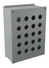
Wiegmann pushbutton enclosure, 20 holes, 30mm, NEMA 12, 14 x 11 x 5in (HxWxD), wall mount, carbon steel, ANSI 61 gray, powder coat finish, screw cover.
