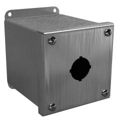
Wiegmann pushbutton enclosure, 1 hole, 30mm, NEMA 4/4X/12/13, 4 x 4 x 5in (HxWxD), wall mount, 304 stainless steel, No. 3 intermediate polished finish, screw cover.
