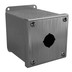
Wiegmann pushbutton enclosure, 1 hole, 30mm, NEMA 4/4X/12/13,  $4 \times 4 \times 5$ in (HxWxD), wall mount, 304 stainless steel, No. 3 intermediate polished finish, screw cover.
